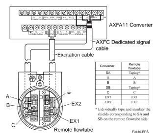
Figure 4.4.6 Wiring Diagram
